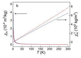
Fig. 2 (a) Magnetization curves of GdF<sub>3</sub>@EG (blue) and GdF<sub>3</sub>@PSSMA nanoparticles (red) at 2 (solid line) and 300 K (dot line) and (b) temperature dependence of mass magnetic susceptibility ( $\chi_m$ ; solid line) and inverse mass magnetic susceptibility of particles ( $\chi_m^{-1}$ ; dot line) measured at cooling in the applied magnetic field of 0.1 T.
