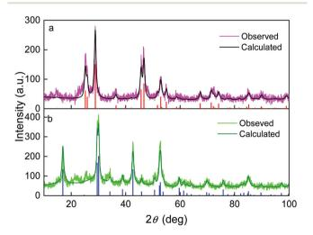
Fig. 1 XRD diffractograms of (a) GdF3@EG and (b) GdF3@PSSMA nanoparticles and comparison with calculated patterns. The vertical lines indicate diffractions of the hexagonal (red) and orthorhombic LnF3 phases (blue). The original data retrieved from Inorganic Crystal Structure Database were based on the P6<sub>3</sub>/mcm of CeF<sub>3</sub> no. 42470 and Pnma of EuF<sub>3</sub> no. 95244 reflected by calculated patterns no. 01-074-3116 and 01-089-1933 in PDF, respectively.
