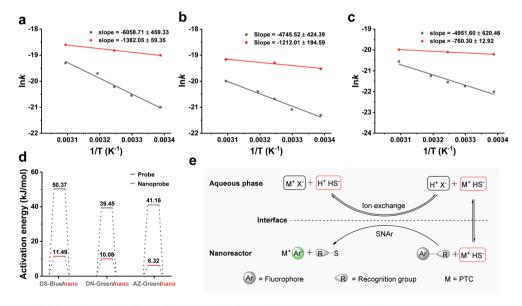
Fig. 4 Kinetic study of DS-Blue-Nano, DN-Green-Nano, and AZ-Green-Nano and proposed PTC mechanism of the nanoreactor to H2S. (a-c) Arrhenius plot of DS-Blue, DS-Blue-Nano, DN-Green, DN-Green-Nano, AZ-Green, and AZ-Green-Nano; (d) The thermal activation energy of DS-Blue, DS-Blue-Nano, DN-Green, DN-Green-Nano, AZ-Green, and AZ-Green-Nano; (e) Proposed PTC mechanism of the nanoreactor in accelerating the reaction of probes to H<sub>2</sub>S.
