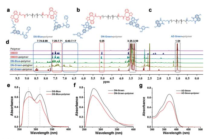
Fig. 2 Synthesis and characterization of probe-polymer conjugates. (a-c) Chemical structure of the fluorescent probe-polymer conjugates, DS-Blue-polymer, DN-Green-polymer, and AZ-Green-polymer. (d) <sup>1</sup>H NMR spectra of polymer, DBCO, DBCO-polymer, DS-Blue-polymer, DN-Green-polymer, and AZ-Green-polymer in DMSO-d<sub>6</sub>. (e-g) Absorbance of DS-Blue, DS-Blue-polymer, DN-Green, DN-Green-polymer, AZ-Green, and AZ-Green-polymer in DMSO.
