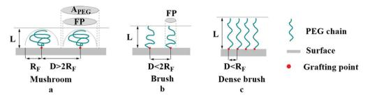
Fig. 4 PEG conformations on a particle surface: (a) Mushroom conformation, (b) brush conformation, and (c) Dense brush conformation. FP: PEG footprint (projected area),  $A_{PEG}$ : area available to each PEG chain. FP =  $A_{PEG}$  in the brush regime, and  $A_{PEG}$  > FP in the mushroom regime.
