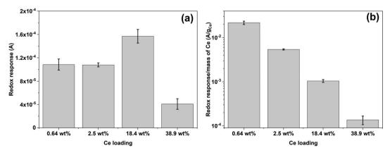
Fig. 6 (a) Redox response obtained with the different CeO<sub>x</sub> nanoclusters/carbon composites toward 10 mM of 'OH (Fenton reaction) and (b) redox response normalized per mass of cerium on the composite. The error bars represent the standard deviation of three repetitive measurements.
