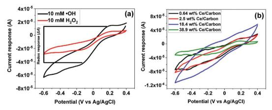
Fig. 5 (a) Calculation example of the current response to hydroxyl radicals and (b) CV results of the sensor response toward 10 mM of 'OH (Fenton reaction) with the different CeO<sub>x</sub> nanoclusters/carbon composites.
