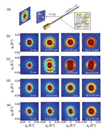
**Fig. 4** (a) Schematic illustration of SAXS experiment. Selected 2D SAXS pattern of (b) GP03-fast, (c) GP03-slow, (d) GP15-fast, and (e) GP03-slow at different holding times.
