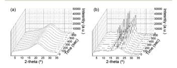
Fig. 3 Development of WAXS profiles as a function of holding time for (a) neat PEG solution and (b) PEG solution with 1.5 wt% GO.
