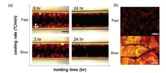
Fig. 2 POM images of (a) GO LC in the polymer solution with different polymer crystallizations and (b) birefringence in the film after complete evaporation. The scale bar is 500 μm.
