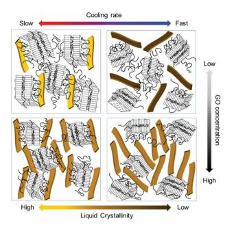
Fig. 7 Schematic images of GO LC with polymer crystal structure cooling at fast and slow speed.
