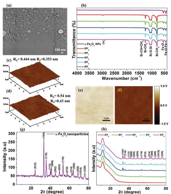
Fig. 2 (a) FESEM view of the PF<sub>2</sub> film and (b) FTIR spectra of  $\alpha$ -Fe<sub>2</sub>O<sub>3</sub> NPs, PDMS, and PDMS@ $\alpha$ -Fe<sub>2</sub>O<sub>3</sub> NP composites; AFM images (three-dimensional) of the (c) PDMS film and (d) PF<sub>2</sub> film; KPFM images of (e) PDMS film and (f) PF<sub>2</sub> film. XRD plots of (g)  $\alpha$ -Fe<sub>2</sub>O<sub>3</sub> nanoparticles and (h) PDMS@ $\alpha$ -Fe<sub>2</sub>O<sub>3</sub> NP composites.
