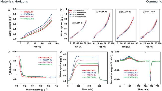
Fig. 3 (a) Water vapor sorption isotherms at 25 °C, (b) water vapor sorption and desorption isotherms at 25 °C and 50 °C, (c) Δ<sub>s</sub>H as a function of water vapor uptake, (d) static water sorption-desorption curves, and (e) 1st derivative curves of static water sorption-desorption for PAETA-X hydrogels.
