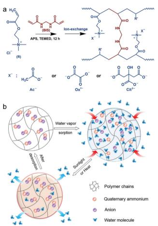
Fig. 1 (a) Schematic illustration of the synthetic procedure of PAETA–X hydrogels paired with  $Cl^-$ ,  $Ac^-$ ,  $Ox^{2-}$ , and  $Cit^{3-}$  counter anions. (b) Schematic illustration of PAETA–X hydrogel with reversible water vapor sorption and desorption properties.
