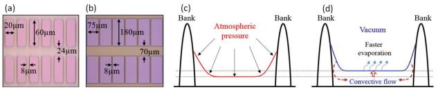
Fig. 19 Image of patterned pixel bank of size (a)  $20 \times 60 \, \mu m$  and  $75 \times 180 \, \mu m$  (b)  $20 \times 60 \, \mu m$  and  $75 \times 180 \, \mu m$ . Schematic view of film formation process under (c) atmospheric pressure and (d) partial vacuum (reprinted with permission from the ref. 102)
