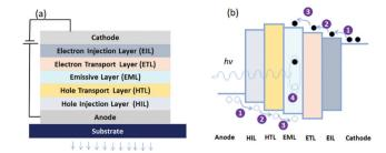
Fig. 2 (a) Multi-layer OLEDs structure, and (b) corresponding energy level diagram.
