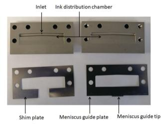
Fig. 6 Schematic of the slot-die head with meniscus guide plate and the shim plate. Image taken in our laboratory.
