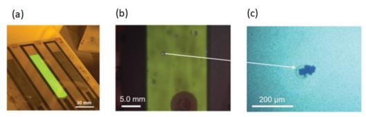
Fig. 10 (a) Image of an OLED with slot-die coated HIL/EML. (b) Overlay of lock-in IR imaging at a bias voltage of 2 V (c) and optical image of dust particle of the slot-die coated OLEDs (reprinted with the permission from the ref. 92).
