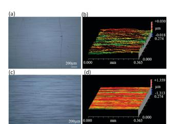
Fig. 21 Surface of head A's (a) optical image and (b) its surface profile. Surface of head B's (c) optical image and (d) its surface profile (reprinted with the permission from the ref. 106).
