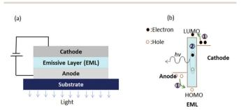
Fig. 1 (a) Schematic of single layer OLEDs, and (b) corresponding energy level diagram.
