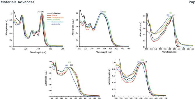
Fig. 5 Absorption spectra of 1 (top left) and AA-DSF-IF (top middle) DD-DSF-IF (top right), DA1-DSF-IF (bottom left) and DA2-DSF-IF (bottom right) in different solvent polarity media: cyclohexane (black line), toluene (red line), chloroform (green line), THF (orange line), dichloromethane (cyan line), and acetonitrile (blue line).
