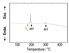
Fig. 2 DTA curve of  $Na_3BS_3$  glass. The orange arrow shows the glass transition temperature, and the two black arrows show the heat-treatment temperatures employed to prepare the glass-ceramics.
