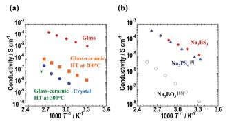
Fig. 6 Temperature dependence of conductivity for (a) Na<sub>3</sub>BS<sub>3</sub> glass, glass-ceramics, and crystal electrolytes and (b)  $Na_3BS_3$ ,  $Na_3BO_3$ ,  $^{13}$  and Na<sub>3</sub>PS<sub>4</sub>,<sup>5</sup> glass electrolytes
