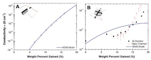
Fig. 7 Conductivity as a function of water content by weight for eumelanin pellets (A) in sandwich and (B) van der Pauw geometries (respectively, insets in (A) and (B)). The solid blue line shows the corresponding MD model. (Reproduced from ref. 114, copyright (2012), American Institute of Physics (AIP)).
