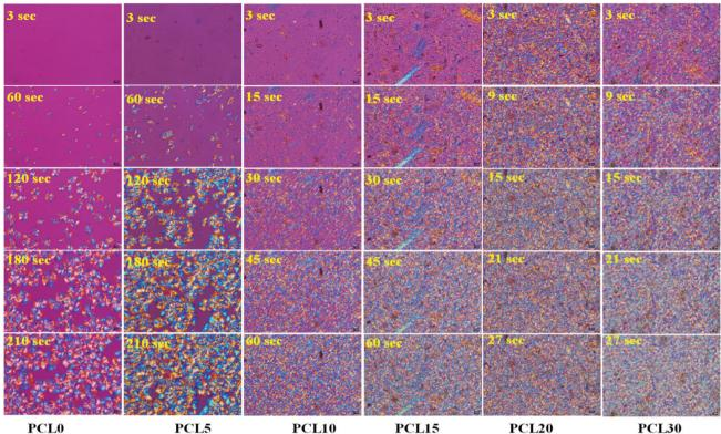
POM micrographs of time-lapse spherulite growth in neat PCL (PCL0) and PCL biocomposites (magnification: 50×).
