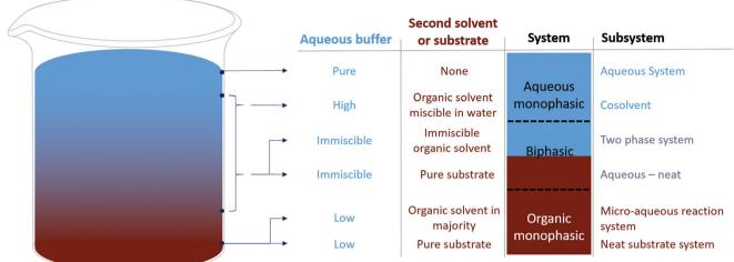
Fig. 1 Scheme of different solvent systems sorted by relative water content.
