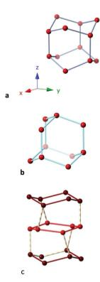
Fig. 19 Fragments of the crystal structure of (a) ice 1 h, 93,103 constituted by boats in the x, and y directions and chairs in the z direction (b) ice Ic with a diamond structure, and (c) ice II,95 showing the chairs formed by each of the two crystallographically independent oxygen atoms, connected vertically forming irregular rings in the perpendicular direction.
