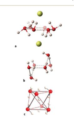
Fig. 17 Structures of hexawater clusters that represent snapshots along the hexagon to octahedron pathway: (a) Planar hexagon (the spheres above and below the O<sub>6</sub> plane represent chloride ions.<sup>97</sup> (b) A chair conformation with a divacant-cube shape, 98 and (c) an octahedron. 98
