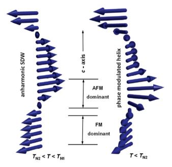
Fig. 5 Schematic representation of the anharmonic spin density wave (SDW) and the phase modulated helix, corresponding to the high-temperature lock-in phase and the ground state of A<sup>2+</sup>Mn<sub>7</sub>O<sub>12</sub> manganites.<sup>4</sup>
