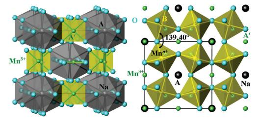
Fig. 1 Crystal structure of the parent cubic modification of A-site-ordered quadruple perovskites  $AMn_7O_{12}$  and  $AA'_3B_4O_{12}$  in space group  $Im\bar{3}$  exemplified by the structure of NaMn<sub>7</sub>O<sub>12</sub> at RT.<sup>12</sup> An Mn-O-Mn (B-O-B) angle is given. A-site polyhedra are shown on the left, and B-site octahedra on the right.
