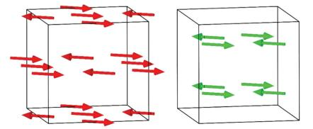
Fig. 7 The A' site ferrimagnetic structure (red, left) and B site C-type antiferromagnetic structure (green, right) observed for R = La, Ce, Nd, Sm, Eu, Dy and Y, and likely common to all  $R^{3+}Mn_7O_{12}$  compounds below  $T_{N1}$ . <sup>59,65,67</sup> The cubes represent the unit cell. The monoclinic b-axis points up the page, and the c-axis to the right.
