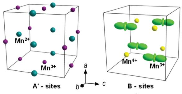
Fig. 4 Charge (left) and orbital (right) ordering in the orthorhombic *Pnn*2 phase of HgMn<sub>7</sub>O<sub>12</sub> perovskite.<sup>39</sup>
