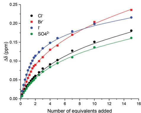
**Fig. 3** Experimental titration data (points) and calculated 1 : 2 host : guest stoichiometric binding isotherms (lines) for the addition of anions as their TBA salts to XB rotaxane **11-PF<sub>6</sub>** monitoring internal macrocycle proton  $\beta$  ( $\text{CDCl}_3/\text{CD}_3\text{OD}/\text{D}_2\text{O}$  45 : 45 : 10, 298 K, 500 MHz).
