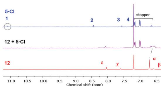
**Fig. 6** Truncated <sup>1</sup>H NMR spectra (400 MHz, CDCl<sub>3</sub>, 298 K) of imidazolium-alkyne **5**·Cl (top), an equimolar mixture of macrocycle **12** and **5**·Cl (middle), and macrocycle **12** (bottom).
