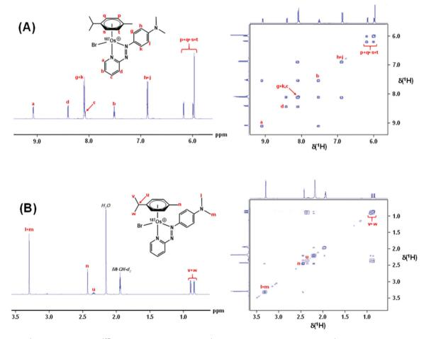
Fig. 3 700 MHz <sup>1</sup>H NMR spectrum of [<sup>187</sup>Os]-1 (LHS), and 400 MHz 2D <sup>1</sup>H COSY NMR spectrum of 1 with all <sup>1</sup>H resonances assigned. (A) The aromatic region, and (B) the aliphatic region. Samples were prepared in MeCN- $d_3$ .
