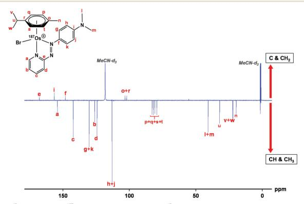
Fig. 5 176 Hz  $^{13}$ C NMR spectrum of  $^{187}$ Os]-1 using the J-MOD sequence, with  $^{13}$ C assignments. The sample was prepared in MeCN- $d_3$ . C and CH<sub>2</sub> peaks are upright, CH and CH<sub>3</sub> peaks inverted.
