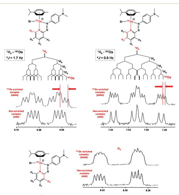
Fig. 4 <sup>1</sup>H NMR (250 MHz) spectra of [<sup>187</sup>Os]-1 compared to natural abundance 1, with expansions of the resonances for <sup>1</sup>H<sub>a</sub>, <sup>1</sup>H<sub>b</sub>, and <sup>1</sup>H<sub>d</sub> illustrating their couplings to other protons and  $^{187}$ Os. Samples were prepared in MeCN- $d_3$ .
