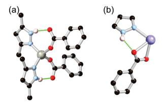
Fig. 2 Two commonly-encountered pyrazole-carboxylate coordination modes involving inter-ligand hydrogen bonding: (a) the  $R_1^{-1}(7)$  motif and (b) the R<sub>1</sub><sup>1</sup>(5) motif. In the former case, the typical D···A distances fall in the range 2.7-2.8 Å with D-H...A angles >150°, while in the latter case these values are more commonly 2.8-2.9 Å and 140-150°, respectively.
