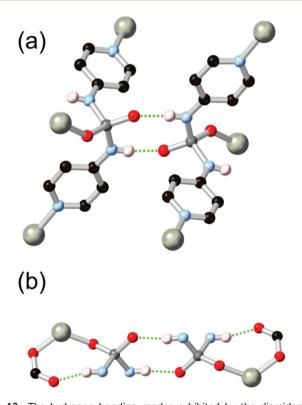
Fig. 12 The hydrogen bonding modes exhibited by the diamidophosphate ligand L21<sup>2-</sup> in a zinc(II) MOF reported by Boomishanker.<sup>98</sup> Adjacent metal sites were linked by an R<sub>2</sub><sup>2</sup>(8) interaction (a), and further supported by an inner-sphere R<sub>1</sub><sup>1</sup>(8) motif (b). The D-A distances are 2.80 and 2.83 Å for formate and diamidophosphate acceptors, respectively, with D-H...A angles of 159 and 172°.
