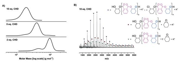
Fig. 2 A) Molar mass distributions for the PA/CHO ROCOP polyester (poly(cyclohexene-alt-phthalate)) [PCHPE] synthesised with complex 1, showing that 10 equivalents of diol (chain transfer agent) are sufficient to yield monomodal molar mass distributions. B) MALDI-TOF spectrum of PCHPE synthesised with 10 equivalents of 1,2-cyclohexane diol (CHD).
