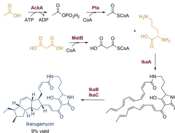
**Scheme 11** Enzymatic total synthesis of ikarugamycin. AckA: acetate kinase; Pta: phosphotransacetylase; MatB: malonyl-CoA synthetase. Starting materials are highlighted in orange. The product is highlighted in blue. Key enzymes in this synthetic route are highlighted in purple. Auxiliary enzymes are highlighted in green.
