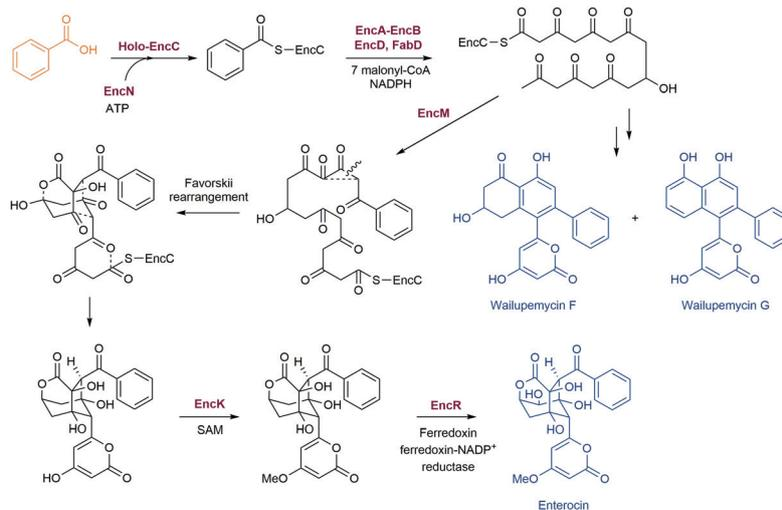
**Scheme 13** Enzymatic total synthesis of enterocin and wailupemycin. Starting materials are highlighted in orange. The products are highlighted in blue. Key enzymes in this synthetic route are highlighted in purple.
