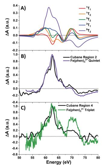
Fig. 4 (A) LFM simulations of cubane excited states, and (B) normalized quintet difference spectra of Fe(phen)<sub>3</sub><sup>2+</sup> (from ref. 22) compared with that of cubane Region 2, and (C) triplet intermediate spectrum (ibid.) compared with cubane Region 4. Fe(phen)<sub>3</sub><sup>2+</sup> spectra have been blue-shifted 5.5 eV.
