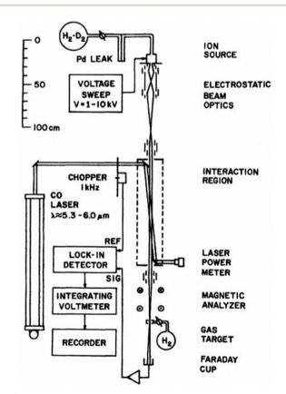
**Fig. 2** Doppler-tuned fast-ion-beam laser spectrometer by Wing and coworkers. Reprinted from ref. 58 with permission of APS.
