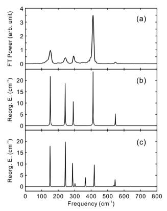
Fig. 8 VSS $_1$  of PM650 obtained by (a) Fourier transform power spectrum and (b) LPSVD. (c) Vibrational reorganization energies calculated by  $S_0-S_1$  displacements by DFT and TDDFT methods using CAM-B3LYP/6-31+G(d,p).
