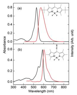
Fig. 1 Absorption (black lines, left axis) and fluorescence (red lines, right axis) spectra of (a) PM597 and (b) PM650 in cyclohexane. Molecular structures of PM597 and PM650 are also shown
