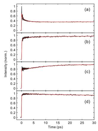
Fig. 4 Time-resolved fluorescence signals of the S<sub>1</sub> state in the longer time range. (a) PM597, 543 nm; (b) PM597, 630 nm; (c) PM650, 586 nm; (d) PM650, 652 nm
