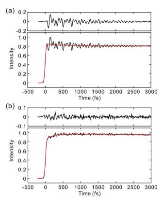
Fig. 3 TF signals of the S<sub>1</sub> state of PM650 in cyclohexane detected at (a) 590 nm and (b) 652 nm. Exponential fits (red lines) are shown together with the residuals
