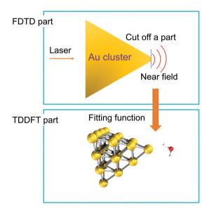
Fig. 4 A schematic diagram showing the mixed FDTD/TDDFT scheme for the PDWS reaction with large-sized NPs.
