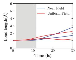
Fig. 6 Time evolution of the OH bonds of Au<sub>20</sub>@H<sub>2</sub>O interacting with the real near field and the uniform electric field, respectively. Here the laser field with  $E_{\rm max}^0 = 0.65 \text{ V Å}^{-1}$  and  $\omega_0 = 3.07 \text{ eV}$  is applied.
