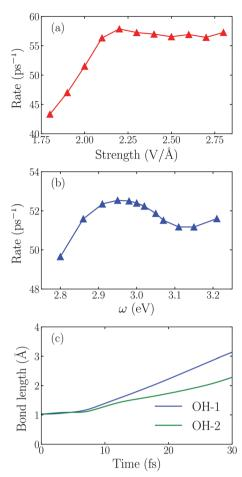
Fig. 3 (a) The reaction rate varies with the intensity of the incident laser with  $\omega_0$  = 3.07 eV. (b) The reaction rate varies with the frequency of the incident laser with  $E_{\text{max}}^0 = 2.00 \text{ V Å}^{-1}$ . (c) The time evolution of two OH bonds under the laser field with  $E_{\rm max}^0$  = 2.80 V Å<sup>-1</sup> and  $\omega_0$  = 3.07 eV.
