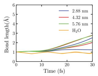
Fig. 5 Time evolution of OH bonds in Au<sub>20</sub>@H<sub>2</sub>O interact with the intensive near field generated by the truncated Au tetrahedron with different side lengths of 2.88 nm, 4.32 nm, and 5.76 nm, respectively. The orange line represents the time evolution of OH bonds in the isolated H<sub>2</sub>O interacting with the near field generated by the whole Au tetrahedron of L = 2.88 nm (without the truncation of  $Au_{20}$ ).
