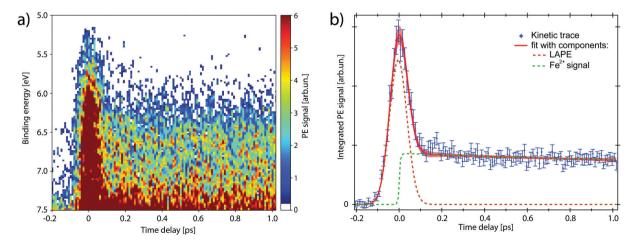
Fig. 4 Time-resolved PE spectra of the ferrioxalate aqueous solution ( $h\nu = 34 \text{ eV}$ ) impulsively excited at 263 nm. (a) 2D map in the energy range where the transient signal and LAPE overlap. (b) Kinetic trace of the transient signal (blue). The fit (red) is plotted with its components: LAPE (orange) and transient signal (green), showing a rise-time much faster than the experimental time resolution (see text for details)
