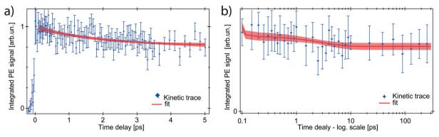
Fig. 5 Kinetic traces of the ferrous PE signal. (a) 5 ps range with LAPE subtracted: a partial intensity drop is observed. The red trace shows the fit with exponentially decreasing component  $A_2$  ( $\tau_2 = 2$  ps). (b) Long-time evolution of the PE signal (up to 250 ps): the ferrous PE signal stabilises to an asymptotic value, which remains for the whole time window.
