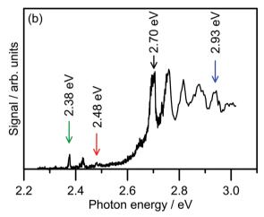
Fig. 2 Photoelectron spectroscopy of 2-Np<sup>-</sup>: (a) example photoelectron spectra; the spectrum in the inset is associated with exciting the dipole-bound state at  $h\nu$  = 2.38 eV, (b) photodetachment spectrum at  $T\approx 300$  K taken from ref. 21. The ADE is 2.4037  $\pm$  0.0005 eV (taken from ref. 23). The feature denoted by \* in the black trace in (a) is attributed to detachment to the ground vibrational state of the 2-naphthoxy neutral  $(^2A^{\prime\prime})$ .
