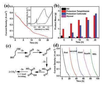
Fig. 3 (a) PET electro-reforming chronoamperometry curve on Pd/NF-10 at 0.7 V vs. RHE; inset: CV curve of the PET electroreforming substrate at a scan rate of 10 mV s<sup>-1</sup>; (b) product analysis of PET electroreforming on Pd/NF-10 at 0.7 V vs. RHE; (c) proposed reaction mechanism for EG oxidation on the Pd/NF-10 electrocatalyst; (d) stability test for PET electro-reforming on Pd/NF-10 at 0.7 V vs. RHE for 5 cycles.
