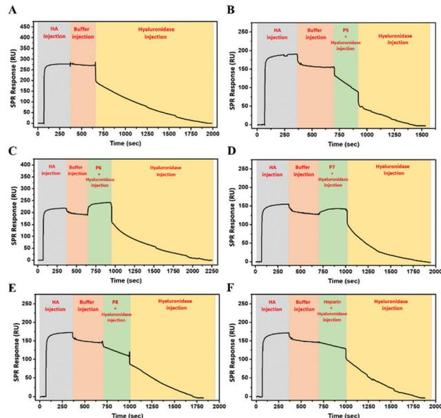
Fig. 6 SPR measurements showing the inhibitory activity of the glycopolymers against hyaluronidase on the degradation of HA bound to the immobilized CD44 receptor; (A) without polymer, (B) **P5**, (C) **P6**, (D) **P7**, (E) **P8**, and (F) heparin.
