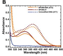
Fig. 2 Dose-dependent photocleavage of NPOM from DNA as monitored in situ by UV-visible absorption spectroscopy. (A) Absorption at 395 nm versus time for NPOM-DNA (AT2, orange) and NPOM-dT nucleoside (brown). Dotted lines indicate single exponential fitting of the data (see also Fig. S1 and S2, ESI†). (B) Absorption spectra of NPOM-DNA (AT2, orange), NPOM-dT (brown), and unmodified DNA duplex (AT1, blue) before (solid line) and after 120 s of light irradiation (dotted line).
