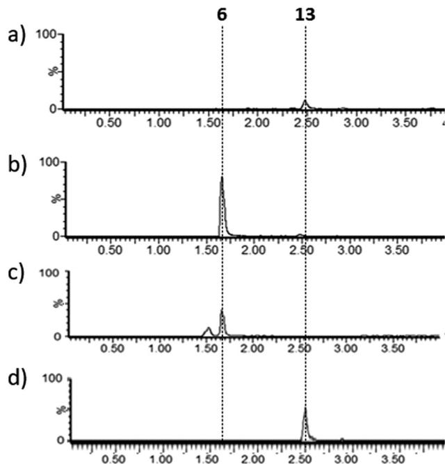
Fig. 6 Extracted ion chromatograms ( $m/z$  154.2 + 288.2) (a) and (b) after incubation of **13** with cell lysates of (a) *E. coli* BL21 or (b) *E. coli* pPigE, (c) synthetic  $H_2$ MAP **6** ( $m/z$  154.16, **6** +  $H^+$ ), (d) synthetic **13** ( $m/z$  288.16, **13** +  $H^+$ ). Retention times corresponding to **6** and **13** are shown.
