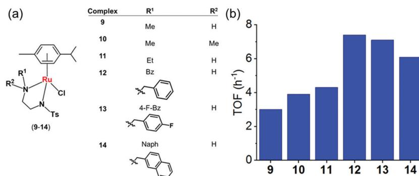
**Fig. 6** (a) Structures of sulfonamidoethylenediamine  $Ru^{II}$  transfer hydrogenation catalysts **9–14**.<sup>22</sup> (b) Turnover frequencies (TOF) for reduction of  $NAD^+$  by formate catalyzed by complexes **9–14**, determined by UV-vis spectroscopy (84  $\mu\text{M}$  complex in MeOH/ $H_2O$  1 : 9 v/v, 102 mM sodium formate and 510  $\mu\text{M}$   $NAD^+$  in  $H_2O$ ).<sup>22</sup>
