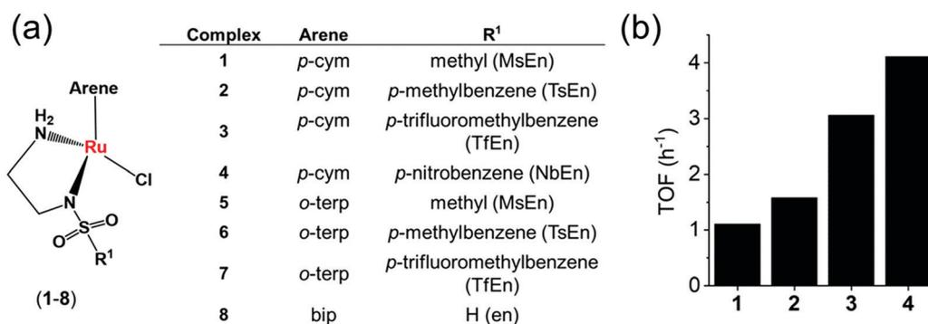
Fig. 4 (a) Structures of sulfonamidoethylenediamine Ru<sup>II</sup> transfer hydrogenation catalysts 1–8.<sup>21</sup> (b) Turnover frequencies (TOF) for NAD<sup>+</sup> reduction in MeOH-d<sub>4</sub>/D<sub>2</sub>O (5 : 1 v/v) by complexes 1–4 determined by <sup>1</sup>H NMR ([Ru complex]: 0.44 mM; [NAD<sup>+</sup>]: 0.88 mM; [formate]: 11.02 mM; molar ratio 1 : 2 : 25).<sup>21</sup>
