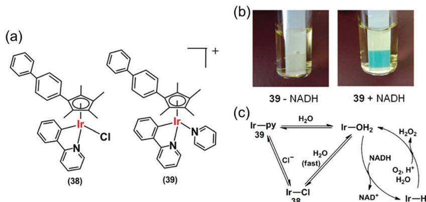
Fig. 12 (a) Ir<sup>III</sup> phenylpyridine transfer hydrogenation catalysts **38** and **39**.<sup>27</sup> (b) Detection of H<sub>2</sub>O<sub>2</sub> in a solution of **39** + NADH in MeOH/H<sub>2</sub>O (3 : 7, v/v) at 310 K by Quantofix peroxide test sticks. (c) Proposed catalytic cycle for the production of H<sub>2</sub>O<sub>2</sub> by **38** and **39**. Reproduced from ref. 27 with permission.
