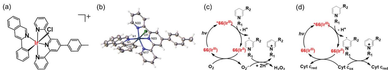
Fig. 17 (a) Line structure, and (b) X-ray crystal structure of photocatalyst complex **66**; the counter ion PF<sub>6</sub><sup>−</sup> is omitted for clarity. Reproduced from ref. 51 with permission. Catalytic cycle for photo-oxidation of NADH by complex **66**; (c) under normoxia, and (d) under hypoxia in the presence of Fe<sup>3+</sup>–cyt *c* as the terminal electron acceptor.<sup>51</sup>
