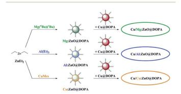
Fig. 3 Overview of M:ZnO@DOPA syntheses and the subsequent combination with Cu@DOPA for the formation of colloidal Cu/ZnO nanocatalysts in hydrogenation of CO<sub>2</sub> to methanol.
