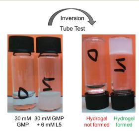
Fig. 3 Gel inversion test.
