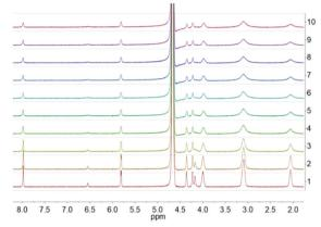
Fig. 7 <sup>1</sup>H NMR spectra recorded during the GMP-**L5** hydrogel formation kinetic studies. Spectra were recorded every 25 seconds. The study was performed employing the optimal conditions for the GMP-L5 hydrogel formation: GMP: L5 5:1 molar ratio.
