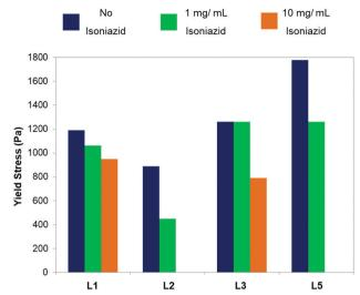
Fig. 9 Yield stress (y) for the GMP-L1, GMP-L2, GMP-L3 and GMP-L5 systems as a function of the isoniazid concentration. The study was performed employing the optimal conditions for hydrogel formation: GMP: L1 3:1, GMP: **L2** 3:1, GMP: **L3** 4:1 and GMP: **L5** 5:1 molar ratios. 10 mg mL<sup>-1</sup> prevented gel formation for the GMP-L2 and GMP-L5 systems.
