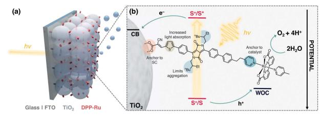
Fig. 1 (a) Schematic representation of the water oxidising dyad-sensitised photoanode. (b) Structure of DPP-Ru with design features and electron transfer events.
