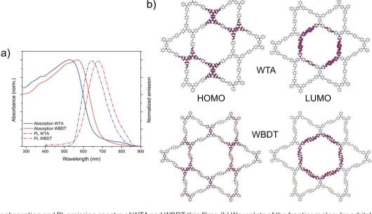
Fig. 4 (a) UV-vis absorption and PL emission spectra of WTA and WBDT thin films. (b) Waveplots of the frontier molecular orbital localizations for WTA and WBDT.
