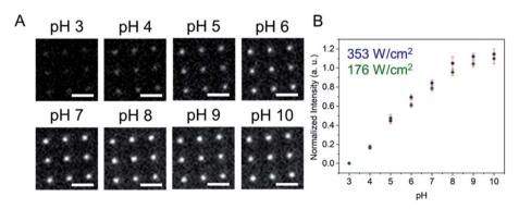
Fig. 2 (A) Wide-field fluorescence images of  $3 \times 3$  E-ZMW arrays containing 3  $\mu$ M fluorescein at different pH values. Scale bars are 2  $\mu$ m. (B) Calibration curve showing  $I_{norm}$  as a function of pH at two laser power densities. Error bars represent the standard deviation of mean values obtained from 9 individual E-ZMW nanopores.
