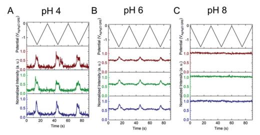
Fig. 4 Applied potential waveform (top) and corresponding individual fluorescence normalized intensity – time traces (bottom) for 3 different E-ZMWs containing 3  $\mu$ M fluorescein. Initial pH values (A) pH 4, (B) 6, and (C) 8.
