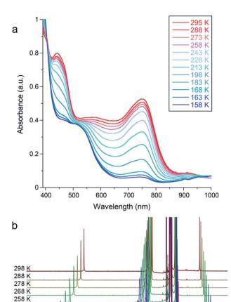
Fig. 3 (a) Variable temperature electronic absorption spectra of 4 in Et<sub>2</sub>O under N<sub>2</sub>. Absorbance values were corrected to account for the change in density of the solvent with temperature. (b) Variable temperature <sup>1</sup>H NMR spectra of 4 in THF-d<sub>8</sub> under N<sub>2</sub>.
