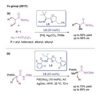
Scheme 10 Chiral acetyl- and Bz-protected aminomethyl oxazoline ligands for the Pd(n)-catalyzed asymmetric C-H functionalization.
