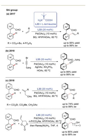
Scheme 40 Pd(II)-catalyzed asymmetric C-H bond functionalization for the construction of axially chiral biaryl aldehydes.
