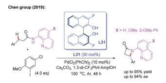
Scheme 35 Pd(II)-catalyzed enantioselective intramolecular  $\beta$ -C(sp<sup>3</sup>)-H amidation of 3-substituted propanamides.
