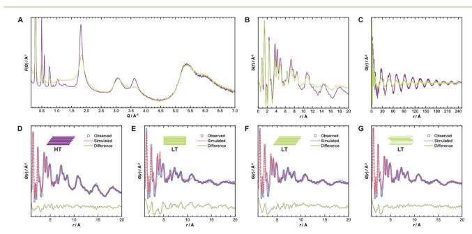
Fig. 5 (A) Comparison of reduced total scattering structure functions F(Q) for HT (purple) and LT (green) collected using synchrotron radiation. (B) Pair distribution functions derived thereof up to 20 Å and (C) up to 250 Å. (D) Best obtained PDF fits over 1–20 Å from structure refinements of HT, assuming unidirectionally slipped stacking, and (E) of LT, assuming eclipsed, (F) unidirectionally slipped, or (G) randomly slipped stacking.
