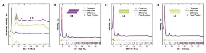
Fig. 4 (A) Comparison of X-ray diffraction patterns of HT (purple) and LT (green) collected with Co  $K\alpha_1$  radiation. (B) Diffraction pattern of HT with best-obtained fit by Rietveld refinement assuming unidirectional slip stacking. (C) Diffraction pattern of LT with best-obtained fit by Rietveld refinement assuming eclipsed stacking and (D) random stacking.
