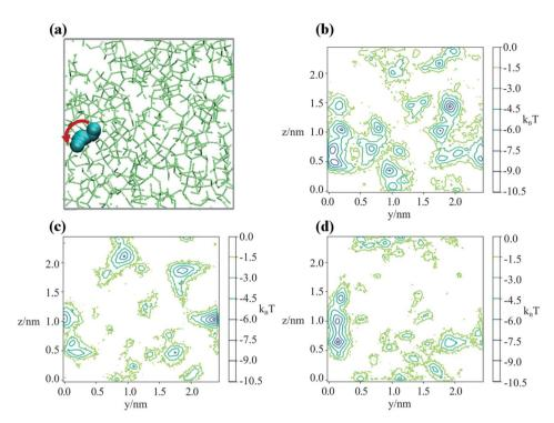
Fig. 3 (a) Snapshots in the yz plane of the trajectory of a water molecule 'jumping' between interstices in an amorphous sucrose lattice. The red arrow indicated the direction of the observed hop. The periodic box is shown in grey. Sequential calculated potentials of mean force that the water experiences are shown in panels (b) to (d), separated in time by 1 ns.
