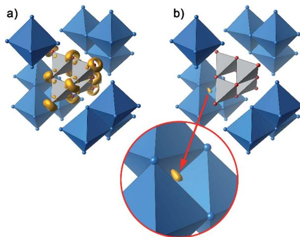
Fig. 8 Selected domains of the electron localization function (ELF): (a) domains in the  $\text{B}_4\text{O}_{10}^{8-}$  anion with  $\eta = 0.84$ , (b) domain with  $\eta = 0.23$  around the attractor in the tetrahedral voids.
