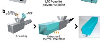
Fig. 3 Fabrication of composite monolithic MOFs. (a) Wash coating to deposit MOFs on monolithic supports. (b) Extrusion approach for the fabrication of monolithic MOFs, with an optical photo of the resulting MOF monolith. Reproduced from ref. 67 with permission from the John Wiley & Sons, copyright 2010.
