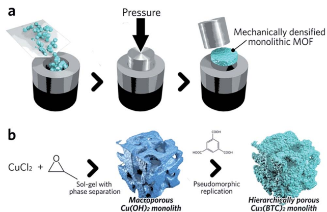
Fig. 4 Schematic of methods available to fabricate single component MOF monoliths. (a) Mechanical densification and (b) coordination replication. (b) is reproduced from ref. 77 with permission from the Royal Society of Chemistry, copyright 2015.
