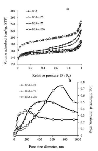
Fig. 5  $N_2$  adsorption-desorption isotherms (a) and Hg-porosimetry (b) of synthesized BEA zeolites.
