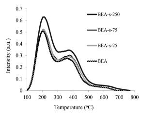
Fig. 7 NH<sub>3</sub>-TPD curves of synthesized BEA zeolites.
