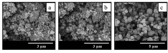
Fig. 1 SEM images of the BEA seed crystals with different SAR: (a) 25; (b) 75; (c) 250
