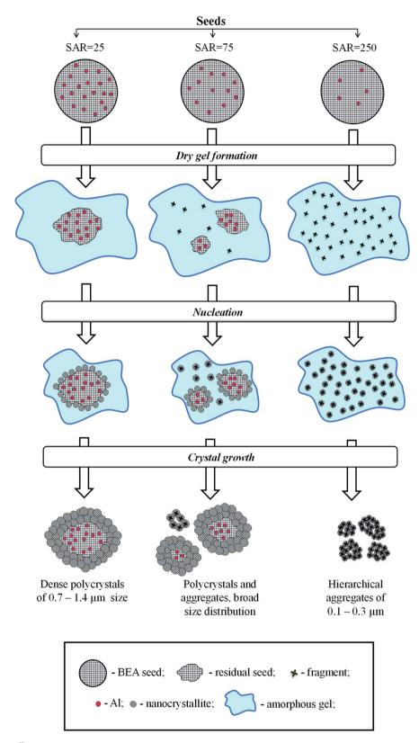
Fig. 6 Mechanism of seeding.
