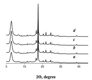
Fig. 2 XRD patterns of synthesized samples: (a) BEA, (b) BEA-s-25, (c) BEA-s-75 and (d) BEA-s-250.
