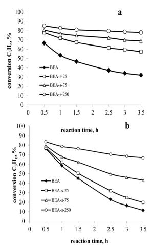
Fig. 8 Propylene conversion *versus* time on stream at 3 MPa, 170  $^{\circ}$ C, WHSV<sub>propylene</sub> = 52 h<sup>-1</sup> and B/P molar ratio of 10 (a) and 5 (b).
