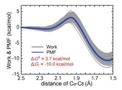
Fig. 4 Work distribution and potential mean force (PMF) obtained for the forced approach between the substrate ( $C_0$ ) and enamine intermediate ( $C_{\alpha}$ ) in DMF solvents, displayed for 0.01 Å ps<sup>-1</sup> for 1000 trajectories in an SMD pulling simulation.
