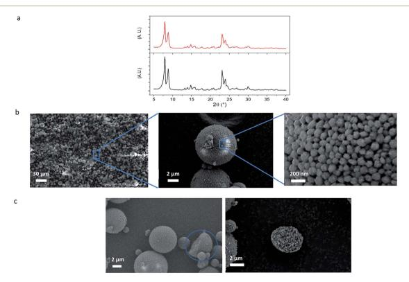
Fig. 2 Characterization of MZM particles. (a) X-ray diffraction pattern for colloidal silicalite-1 (black line) and silicalite-1 MZM (red line), (b) SEM images of the obtained silicalite-1 MZM spherical particles, and (c) cracked silicalite-1 MZM particles.
