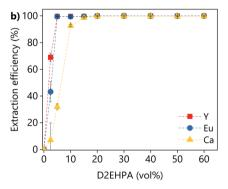
Fig. 14 Effect of the D2EHPA concentration on the extraction efficiency from (a) LevA-ChCl-based PLS or (b) levulinic acid PLS.
