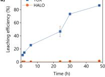
Fig. 7 Effect of the mixing time on the leaching efficiency of a synthetic lamp phosphor mixture using (a) LevA–ChCl and (b) levulinic acid. The leaching conditions are:  $H_2O$  vol% = 30; T=80 °C; L/S = 10; 500 rpm.
