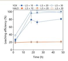
Fig. 10 Effect of the L/S ratio and leaching time on the leaching efficiency of a real lamp phosphor waste using the ionic liquid [Hbet]  $[NTf_2]$ . The leaching conditions are:  $H_2O$  vol% = 5; T = 80 °C; 500 rpm.
