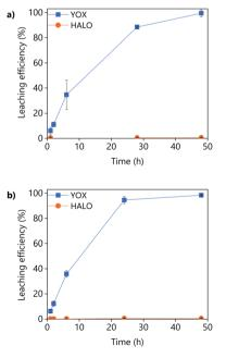
Fig. 5 Effect of the leaching time on the leaching efficiency of YOX and HALO using (a) LevA–ChCl and (b) levulinic acid. The leaching conditions are: T = 80 °C; L/S = 10; H<sub>2</sub>O vol% = 30; and 500 rpm.
