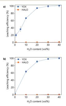
Fig. 4 Effect of the water content on the leaching efficiency of YOX and HALO using (a) LevA–ChCl and (b) levulinic acid. The leaching conditions are:  $T=80\,^{\circ}\text{C}$ ,  $t=48\,\text{h}$ , L/S = 10 and 500 rpm.
