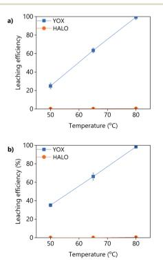
Fig. 6 Effect of the temperature on the leaching efficiency of YOX and HALO using (a) LevA–ChCl and (b) levulinic acid. The leaching conditions are:  $H_2O$  vol% = 30; t = 48 h; L/S = 10; 500 rpm.
