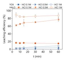
Fig. 11 Effect of the leaching time and HCl concentration on the leaching efficiency of real lamp phosphor waste using an aqueous solution of HCl. The leaching conditions are: T=25 °C; L/S = 10; 500 rpm.
