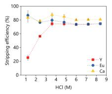
Fig. 15 Effect of the HCl concentration on the stripping efficiency. The stripping conditions were: A/O = 1; mixing time = 30 min, T =
