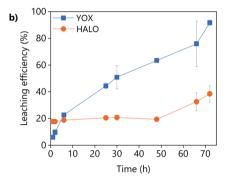
Fig. 8 Effect of the leaching time on the leaching efficiency of a real lamp phosphor waste using (a) LevA-ChCl and (b) levulinic acid. The leaching conditions are:  $H_2O$  vol% = 30; T = 80 °C; L/S = 10; and 500 rpm.
