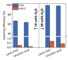
Fig. 3 Comparison of leaching efficiency of YOX and HALO using LevA–ChCl and levulinic acid. The leaching conditions are:  $T = 80 \,^{\circ}$ C,  $t = 48 \, \text{h}$ , L/S: 10 and 500 rpm.
