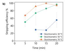
Fig. 12 Stripping efficiency obtained by the addition of pure oxalic acid to (a) LevA-ChCl and (b) levulinic acid PLS, as a function of the amount of oxalic acid, mixing temperature and time. The leaching conditions are:  $H_2O \text{ vol}\% = 30$ ;  $T = 80 \,^{\circ}\text{C}$ ;  $t = 48 \,\text{h}$ ; L/S = 10; 500 rpm.
