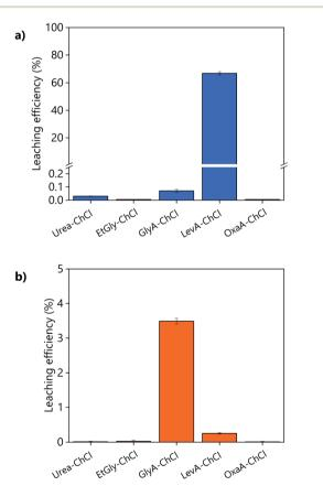
Fig. 2 Effect of the hydrogen-bond donor type on the leaching efficiency of (a) YOX lamp phosphor and (b) HALO lamp phosphor. The leaching conditions are: H<sub>2</sub>O vol% = 10; T=80 °C; t=48 h; L/S = 10 and 500 rpm.
