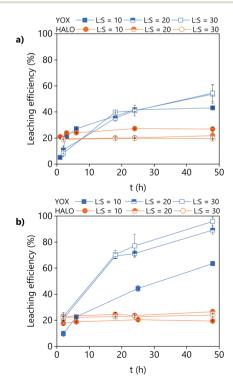
Fig. 9 Effect of the L/S ratio and leaching time on the leaching efficiency of a real lamp phosphor waste using (a) LevA-ChCl and (b) levulinic acid. The leaching conditions are:  $H_2O$  vol% = 30; T = 80 °C; 500 rpm.
