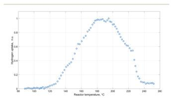
Fig. 5 Hydrogen uptake (normalized units) as a function of reactor temperature during catalyst activation (ambient pressure; inlet gas flowrate 250 N ml min $^{-1}$ ; inlet gas composition: 20 mol% H<sub>2</sub> and 80 mol% N<sub>2</sub>).
