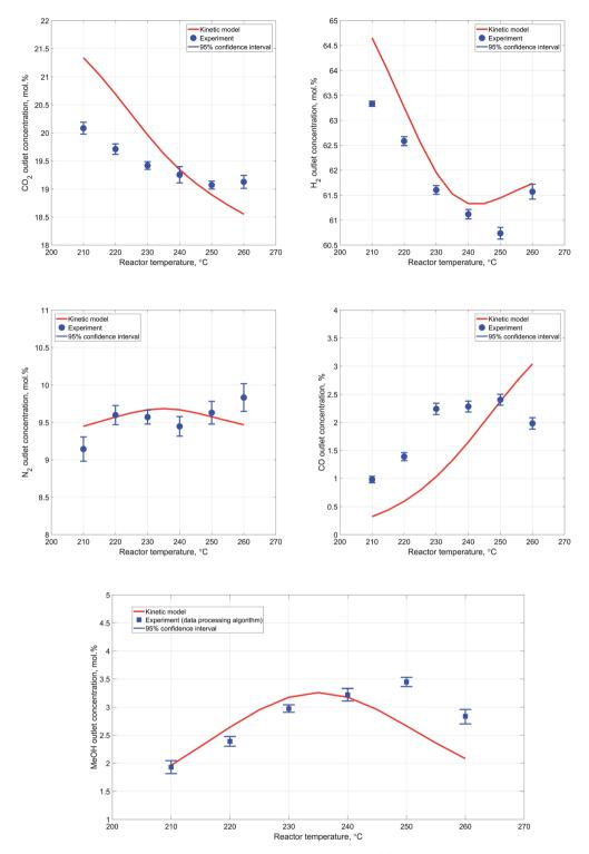
Fig. 8 (a). Dependence of the outlet  $CO_2$  concentration from the reactor temperature. (b) Dependence of the outlet  $H_2$  concentration from the reactor temperature. (c). Dependence of the outlet  $N_2$  concentration from the reactor temperature. (d). Dependence of the outlet CO concentration from the reactor temperature.
