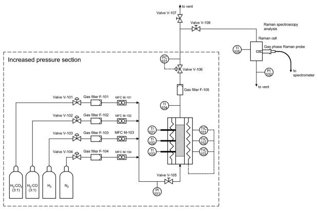
Fig. 1 Flowchart of the reactor system.
