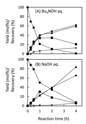
Fig. 5 Changes with time in recovery of LM2 ( $\bigcirc$ ), yields of guaiacol ( $\spadesuit$ ), vanillin ( $\triangle$ ), vanillic acid ( $\bigstar$ ), and enol ethers EEs<sup>a</sup> ( $\bigcirc$ ) during degradation of LM2 (5.0 mg) at 120 °C under air in 1.25 mol L<sup>-1</sup> Bu<sub>4</sub>NOH aq. (1.0 mL) (A) and in 1.25 mol L<sup>-1</sup> NaOH aq. (1.0 mL) (B). <sup>a</sup> The yields of EEs are shown as the sum of the *cis*- and *trans*-isomers.
