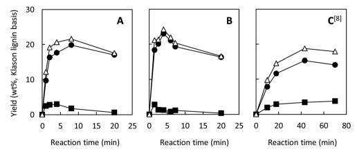
Fig. 1 Changes with time in yields of vanillin ( $\blacksquare$ ), vanillic acid ( $\blacksquare$ ), and their total yields ( $\triangle$ ) during degradation of Japanese cedar wood flour (14 mg) in 1.25 mol L<sup>-1</sup> Bu<sub>4</sub>NOH aq. (2.0 mL) under O<sub>2</sub> (A), under O<sub>2</sub> with the addition of NaOH(s) (200 mg) (B), and under air<sup>8</sup> (C) at 120 °C. The total amount of Klason lignin and acid-soluble lignin of the wood flour was 34.3 wt%.
