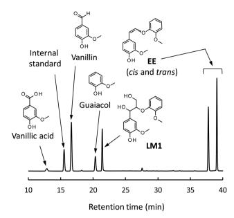
Fig. 4 HPLC chromatogram of the reaction mixture obtained after the degradation of LM2 (5 mg) in 1.25 mol L $^{-1}$  Bu<sub>4</sub>NOH aq. (1.0 mL) under air for 1 h.
