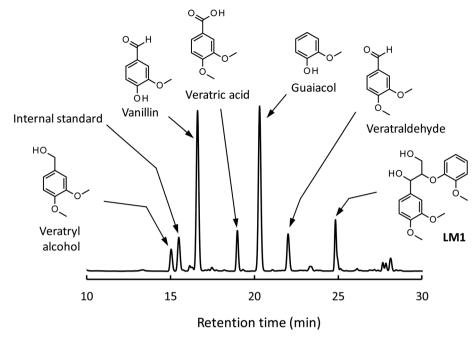
Fig. 2 HPLC chromatogram of the reaction mixture obtained after the degradation of LM1 (20 mg) in 1.25 mol L<sup>-1</sup> Bu<sub>4</sub>NOH ag. (2.0 mL) under air for 4 h.
