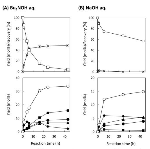
Fig. 3 Changes with time in recovery of LM1 ( $\square$ ), yields of guaiacol ( $\times$ ), veratraldehyde ( $\bullet$ ), vanillin ( $\square$ ), veratric acid ( $\triangle$ ), veratryl alcohol ( $\bullet$ ), and the total yield of the A-ring-derived products ( $\bigcirc$ ) during degradation of LM1 (20 mg) at 120 °C under air in 1.25 mol L<sup>-1</sup> Bu<sub>4</sub>NOH aq. (2.0 mL) (A) and in 1.25 mol L<sup>-1</sup> NaOH aq. (2.0 mL) (B).
