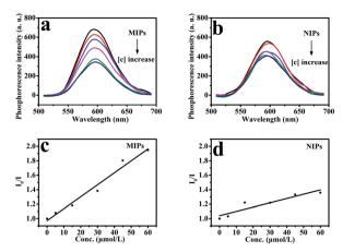
Fig. 9 (a) The RTP emission spectra of Mn-doped ZnS QD@MIPs (45 mg  $\rm L^{-1}$ ) and (b) Mn-doped ZnS QD@NIPs (45 mg  $\rm L^{-1}$ ) with addition of different concentrations of phenol in DDW. The Stern–Volmer values for (c) Mn-doped ZnS QDs@MIPs and (d) Mn-doped ZnS QDs@NIPs.
