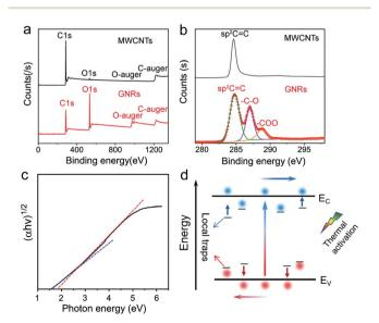
Fig. 3 XPS spectra of MWCNTs and GNRs: (a) full spectra, (b) fine spectra of carbon. (c) Plots of  $(\alpha h \nu)^{1/2}$  against the photon energy in UVvis absorption spectrum of GNRs. (d) Mechanism schematic diagram demonstrating thermal response of GNRs.
