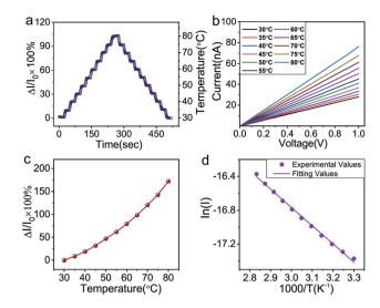
Fig. 4 (a) Step-like curve with the variation of temperature of the GNRs sensor. The right y-coordinate is corresponding temperature of normalized current change. (b) I-V curves of the sensor from 30–80 °C. (c) Plot of normalized current change versus temperature. (d) showing linear relationship between  $\ln(I)$  and 1000/T.
